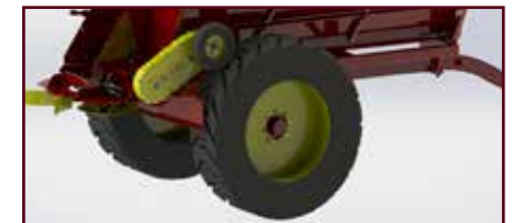
High Flotation Wheels , Durable Imported Axels & Detachable Axel
