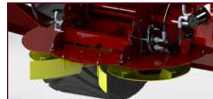
Adjustable high-performance Hydraulic Spinner Motors & Side Mounted Spinner Motors
