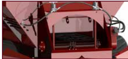
Door width of 1000mm, Adjustable Sleuth Gate & a Robust Chain Conveyor System
